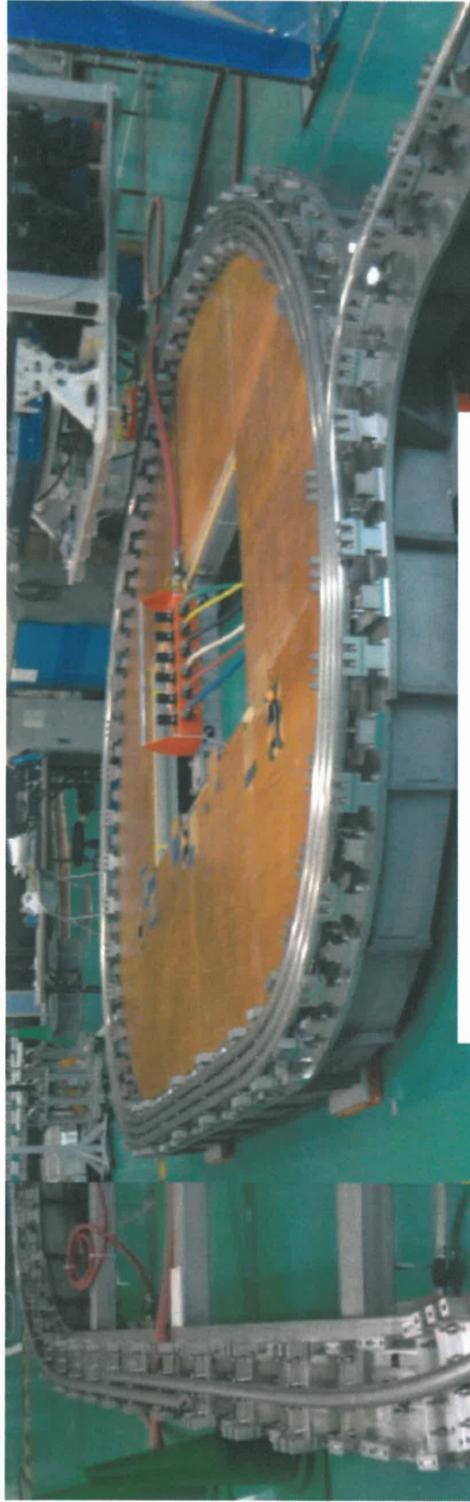
**Completed one third scale 3-turn winding trials at Toshiba**
